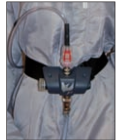
Pressure reducer valve and activated carbon filters
