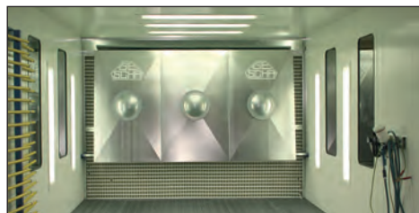
Spray booth with integrated lamps
