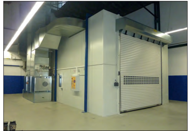
Combination cabin with heat recovery
