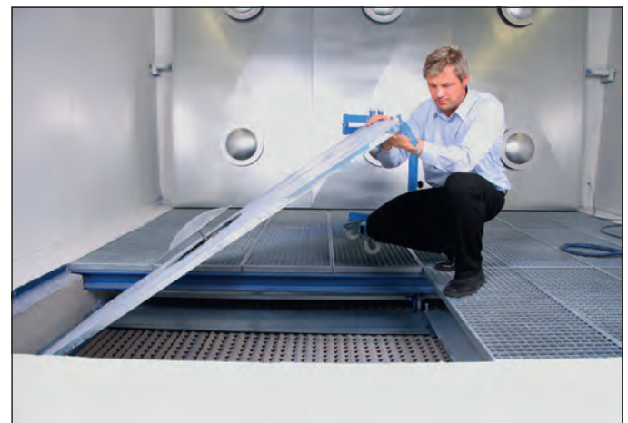
Fast filter exchange system
