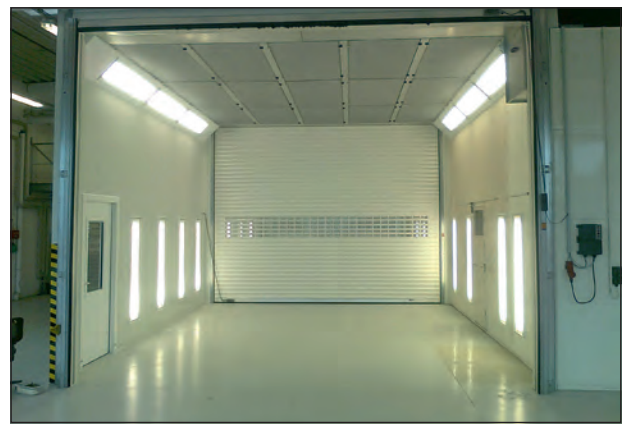
Large area filter with fast exchange system
