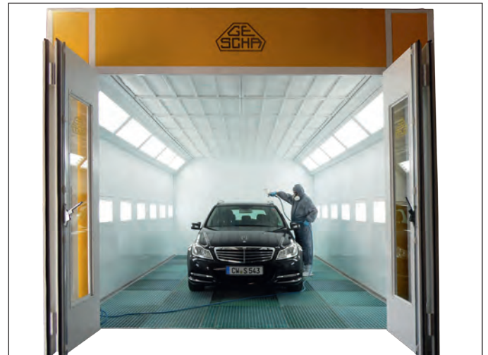
special spray booth with lift and high air speed nozzle
