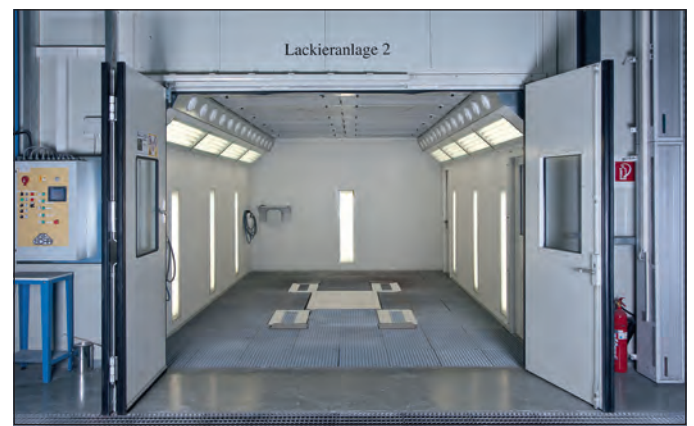
Special spray booth with lift and high air speed nozzles
