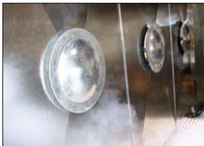
Pre-Paint collector: Our metal front cover already collects a big amount of spray mist, which therefore does not even get to the paint arrestor
